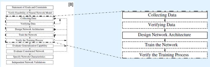
Fig. 2 The development cycle of a neural network
